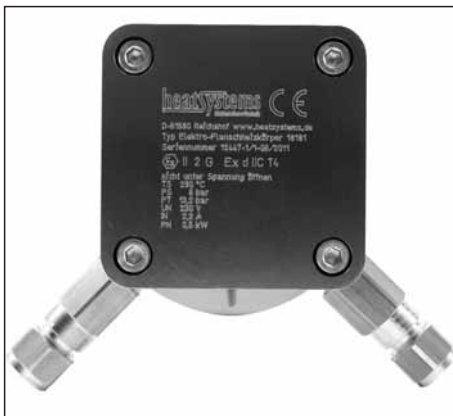
Electric flange heater DN 40 2000 W, dead-leg-free version, for heating of gas.
