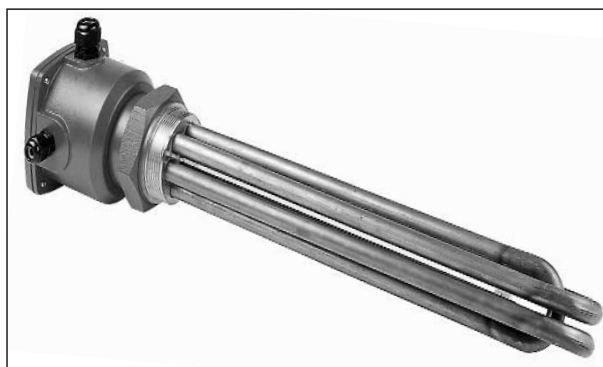
Screw-in heater for medical baths. Heater made of stainless steel Incolloy 825 (2.4858), welded into screw connection made of stainless steel AISI 316L (1.4404/1.4435).
