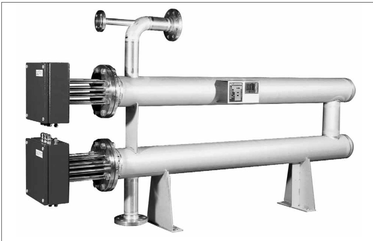
Steam superheater consisting of two flow pipes with built-in electric flange heaters. Operating pressure 10 bar (o), operating temperature 250 °C. Capacity 160 kW.
