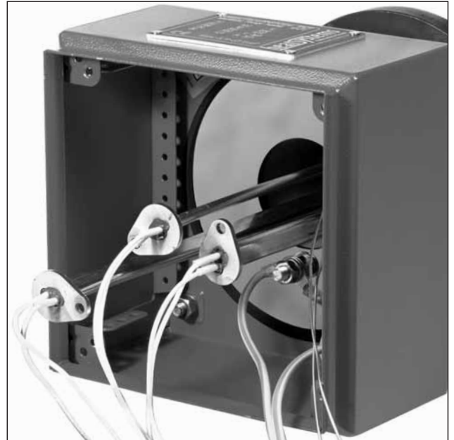
Electric flange heater with exchangeable oval pipe heaters (the heating element can be exchanged without draining the medium).
