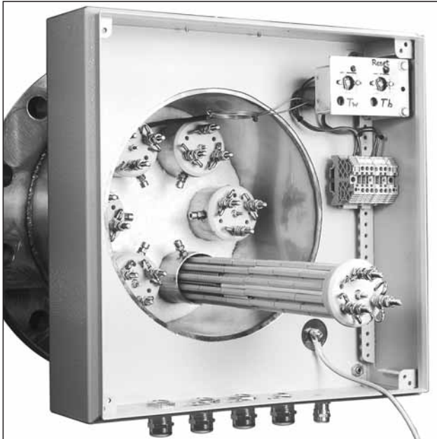
Ceramic heating element with stainless steel protective pipe (the cartridge heater can be changed without draining the medium).
